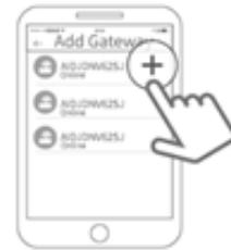
If the connection fails, unplug the Gateway and repeat the process.
